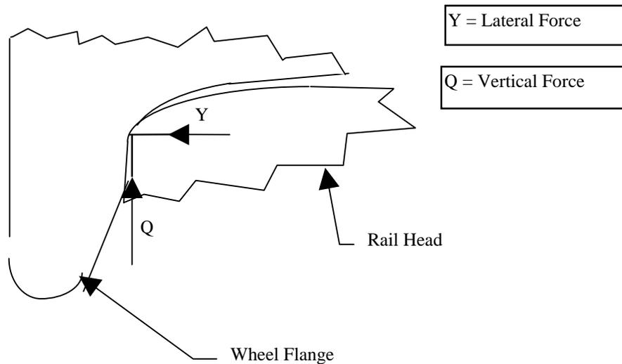
Figure 1. A wheel in flange contact
