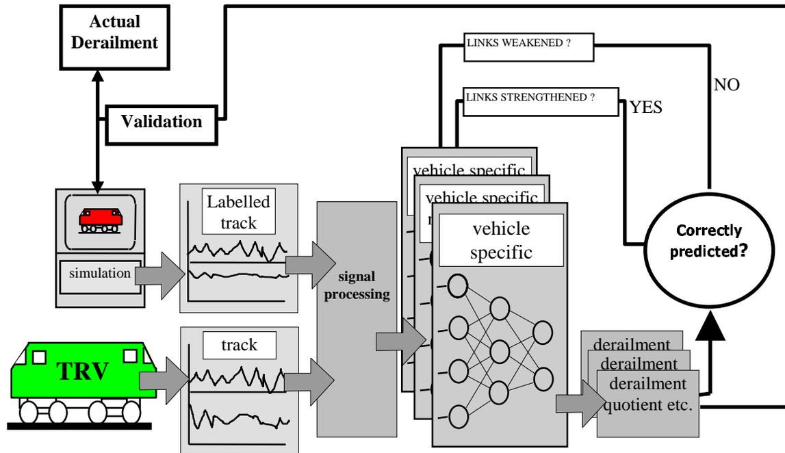
Figure 5. The proposed intelligent track monitoring system
