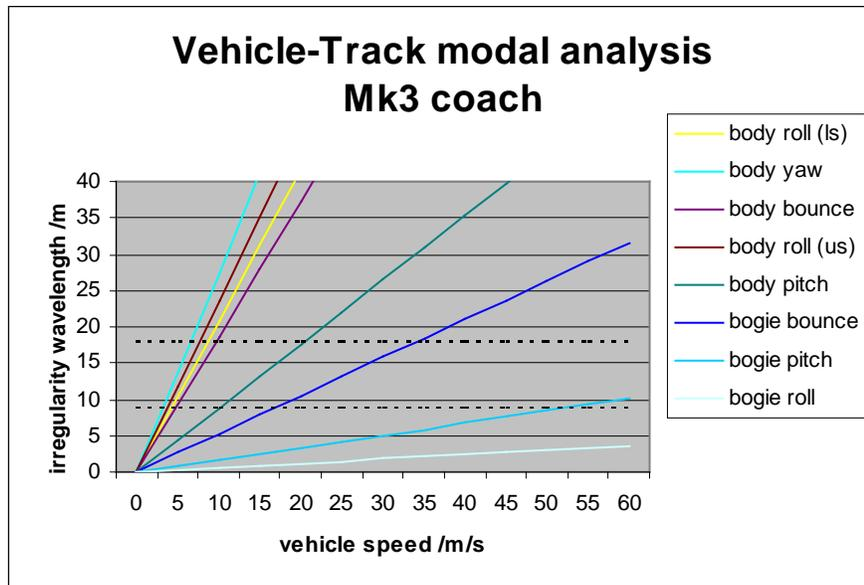
Figure 3. Vehicle modes of oscillation
