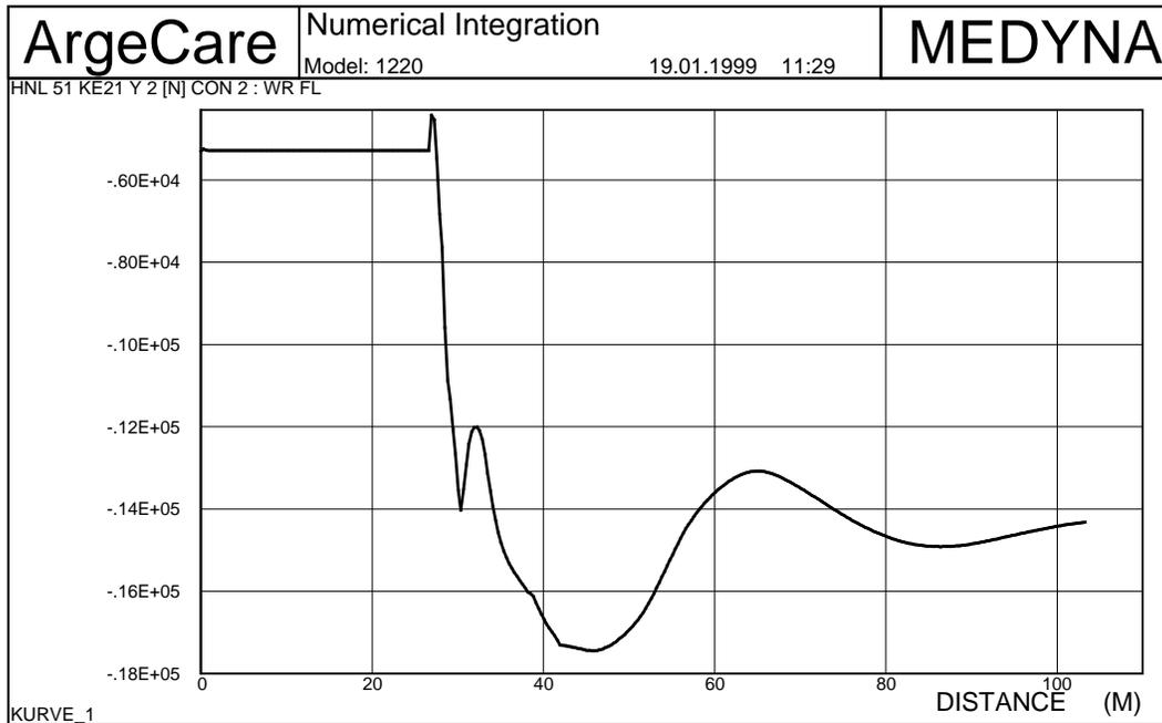
Figure 4. Lateral force on a wheel entering a switch
